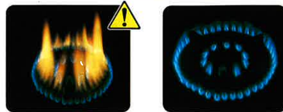
Incomplete combustion (Inadequate air)
